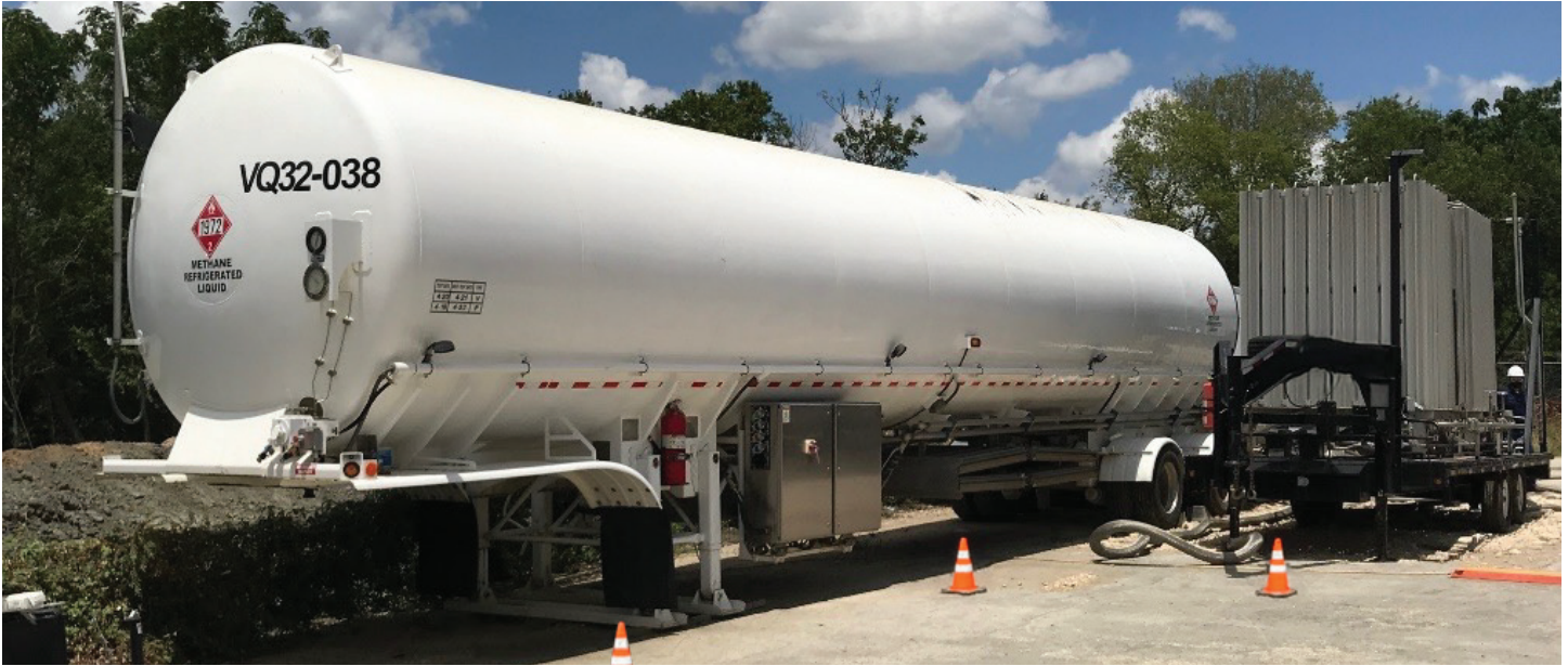
Liquefied Natural Gas (LNG) fueling trailer with ~5,000 LNG gallons of fuel + liquid vaporizer to convert gas to liquid.
